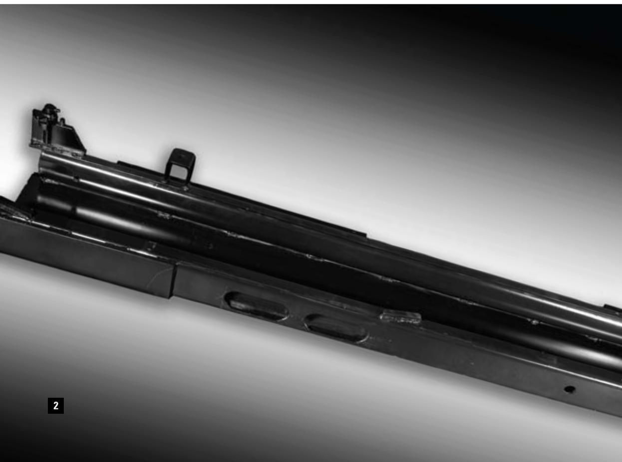
**Convex column surfaces that mate with concave roller assemblies self-center and balance the load without introducing additional torque into the assembly.**
