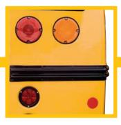
LED clearance lights, direction lights and stop lights are standard equipment offering enhanced safety, while reducing operating and maintenance costs.
