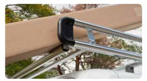
Rear Roller makes loading and unloading easy
