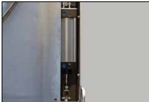
Dual air tailgate cylinders standard
