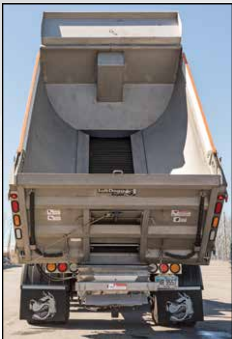
Unique, roll-formed sides and cross member-less design
