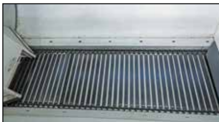
30.25" wide conveyor with 1/2" bars
