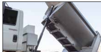
Mailhot® multi-stage, double-acting, nitrated cylinder, trunnion-mounted hoist
