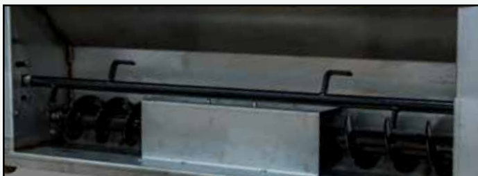
5" Dia. Auger and mixing tines (535000)
